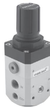
It has the function of regulating the negative vacuum pressure, keeping it stable at set value regardless of flow and variations in the degree of vacuum in the primary network. The units are of a double diaphragm construction and have been designed to exploit to their advantage any existing pressure differential between the
