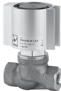
The valves are composed of a bronze body, 2 ways, with pneumatic control, with a compact single or double acting cylinder with connections which can be turned 360°. Versions are available that have the gaskets in contact with the fluid, and are made of NBR, FPM or PTFE.
