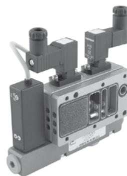
They have been designed to be enclosed between the cap and the base of the “SE” vacuum generator and attached to the latter via M4 screws; with the distribution manifold inside the generator, the compressed air is distributed without having to use external manifolds.
